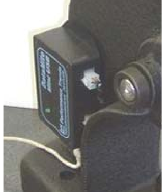
Figure A16 New, 12 Bit Mini Logger (looks same from outside as previous logger)
